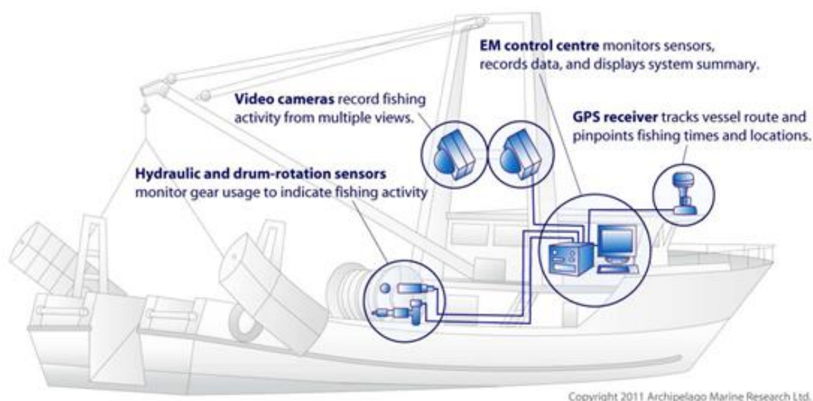
Figure 2: Electronic Monitoring System (Courtesy of Archipelago Marine Research Ltd)
