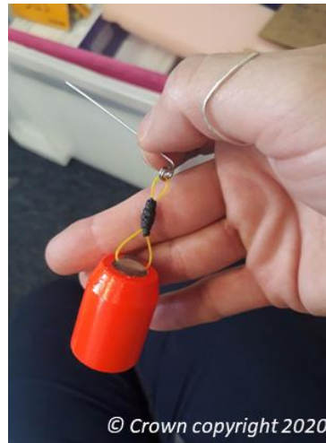
Figure 2.2: Example of the set up with monofilament and crimp for the G5 (20 bar) used during this project.
