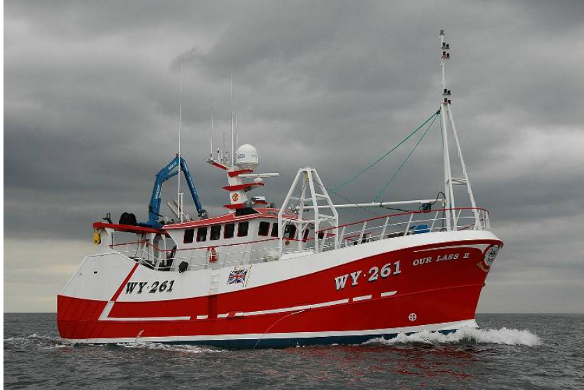
MFV Our Lass II (WY 261) skippered by James Locker Main engine power 480 kW, vessel length 21.5m, home port Whitby
