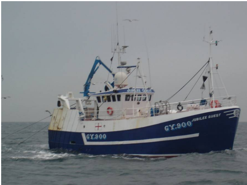
MFV Jubilee Quest (GY 900) skippered by Graham Hall Main engine power 347 kW, vessel length 21.1m, home port Grimsby
