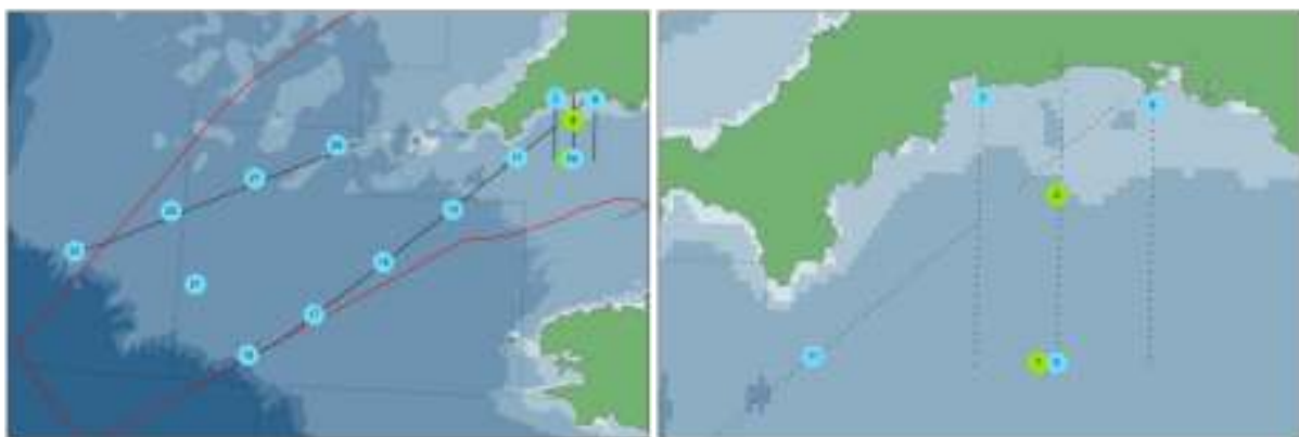
Figure 5. Overview of the survey (left) with detail of Plymouth Bay (right) showing the acoustic transects (black dotted lines), plankton/CTD stations (blue) and fishing stations (green).
