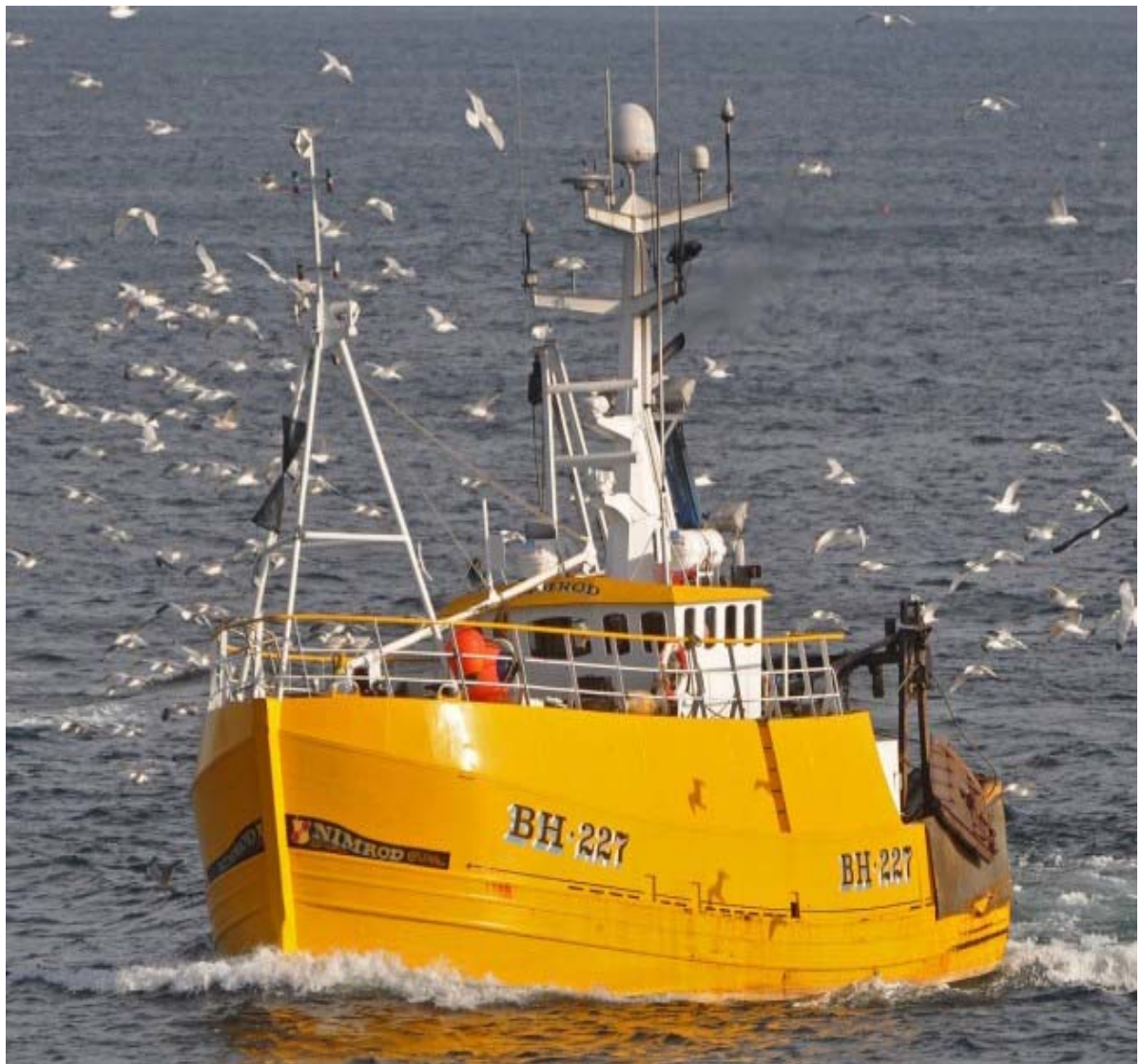
Figure 2.1.1: Nimrod BH227, L.O.A. 15.5m, NT 40.5, 289KW.
